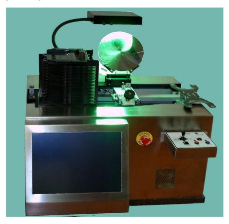
The system is computer controlled, and its use and programming is really easy and user friendly. It is possible, if needed, to edit and recall recipes, and each recipe includes inspection strategies (all wafers, fixed wafers and random access for statistical inspection) and handling parameters.
