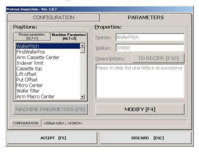
The parameter section is divided into two sections: RECIPE PARAMETERS and MACHINE PARAMETERS.
